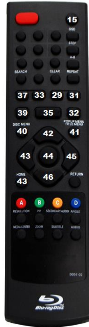
Image for RS485 Control Reference with command number layover for available commands. Buttons without numerical overlays in the above image do not have available RS485 Commands.
