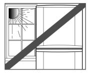
DO NOT expose the fridge/ freezer to direct sunlight. DO NOT install it next to a source of heat (oven, radiator). If you must install the fridge/ freezer near a source of heat, ensure that there is sufficient insulation between the two appliances.
