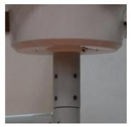
If the head is drifting, or if the movement of the arm is stiff, use a hex tool as indicated in section 4.6 of this manual to tighten the arms.
