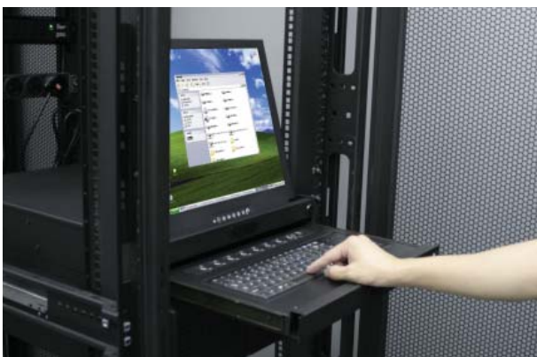
Figure 7. Operating the LCD keyboard drawer.
