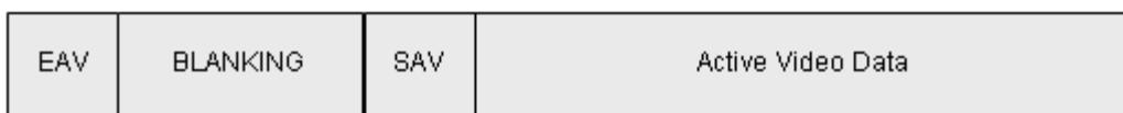
Figure 26: Standard ITU-R BT.656 data stream format for a single horizontal line of digital video data.
