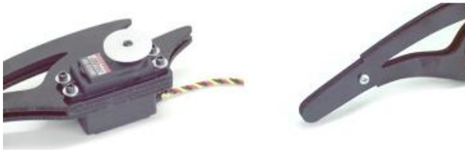
Figure 46: Screws to fasten motor and leg from www.LynxMotion.com (reprinted w/ permission)
