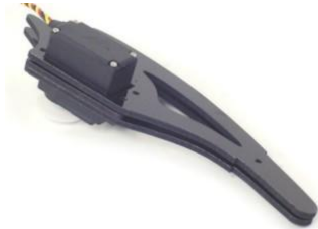
Figure 45: Servo locked by leg structure from www.LynxMotion.com (reprinted w/ permission)
