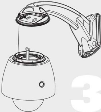
④ Line up the mold lines and assemble main body to Wall Mount Bracket.
