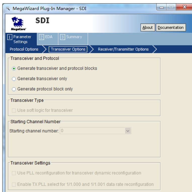
Figure 5-26 Configurations of SDI IP core 2
