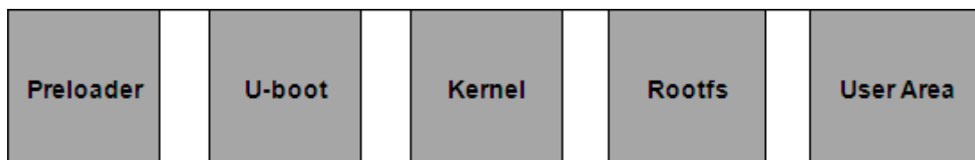
Figure 4-1 Embedded Linux system structure
