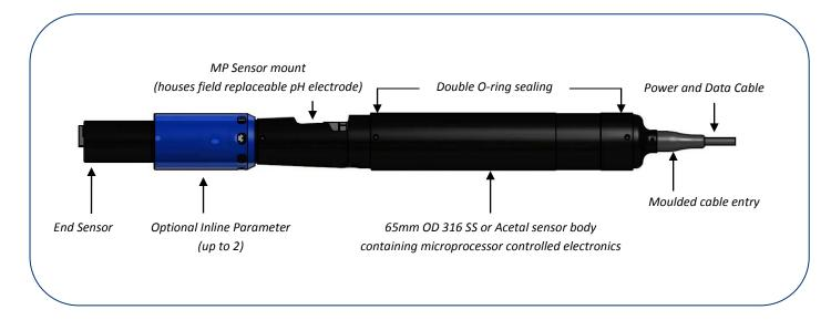
The Greenspan MP47 Sensor consists of the following primary elements:
