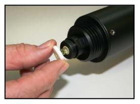
The reference protection ring can be removed and/or replaced (with the electrode still in place in the sensor) by unscrewing the plastic shroud on the end of the electrode. The white protection ring can be slid off the glass electrode.
