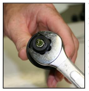
Take care when handling the pH electrode, that it is not handled by the gold contacts. Contamination of this area may degrade the performance and expected life of the electrode
