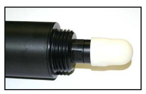
PH electrodes should be stored in such a way to prevent the electrode from drying out. A rubber cap is provided with the electrode for this purpose. A small amount of liquid should be placed in this cap prior to the cap being placed over the electrode. 3M KCl is the preferred storage solution however; tap water should be used if not available. Soaking in pH 4 buffer solution overnight may restore some electrodes that have been allowed to dry out,
