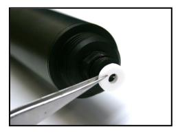
The reference protection ring can be removed and/or replaced (with the electrode still in place in the sensor) by unscrewing the plastic shroud on the end of the electrode. The white protection ring can be slid off the platinum electrode.
