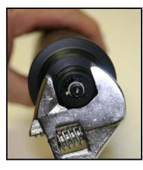
ORP electrodes will require periodic replacement. How long they last is dependent on the environment and to a lesser extent the cleaning and maintenance. In a typical environment, electrode life between 1 and 3 years is quite possible. The electrode is sealed in its mount with two O-rings on the electrode body. The electrode is removed by unscrewing it from the housing. Spanner flats are machined on the electrode to assist.
