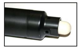
The MP sensor (with pH or ORP) is shipped with a rubber cap covering the electrode. This cap contains a small amount of 3M KCl solution and is in place to prevent the electrode from drying out during shipping and storage. **This cap must be removed prior to installation.** The cap should be retained so that it can be placed back on the electrode if the sensor is to be removed.
