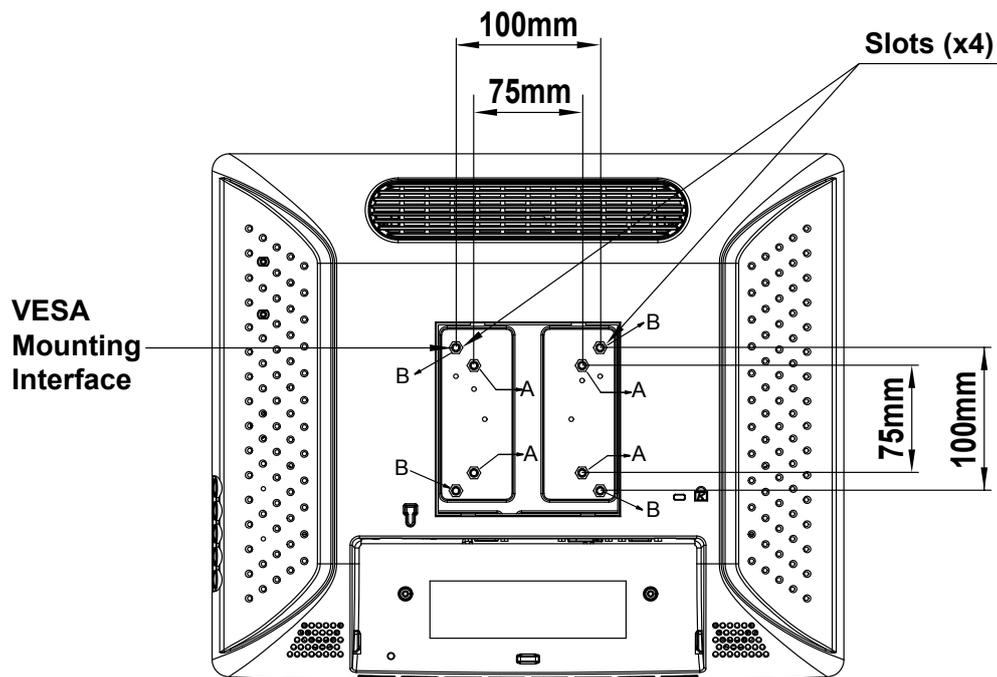
**\*A/B:** The distance between the shielding surface and the bottom of the screw hole is 8 mm.
