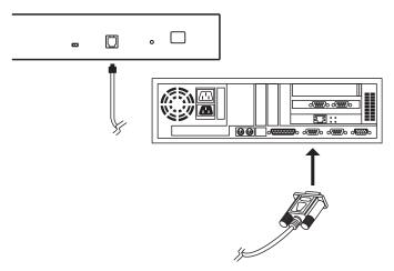
**Note:** On a daisy chained installation, connect the cable to the first station (master) unit. The chained stations (slaves) that are the same model will receive the upgrade via the daisy chain cables.
