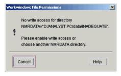
[Cancel] removes the popup window. Directory permissions can only be changed by the directory owner or a user with system privileges. To manually add write permissions to a directory (e.g., \$NMR-DATA/INADEQUATE), type the following command from the NMRanalyst UNIX Shell window:
