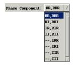
A phase-insensitive 2D spectrum consists of two, a phase-sensitive 2D spectrum of four, and a phase-sensitive 3D spectrum of eight phase components. NMRanalyst spectra contain these phase components. The phase component to be plotted can be selected from this menu. In the menu label, R stands for the real part containing the absorption mode signals after phasing. Label I stands for the imaginary part containing
