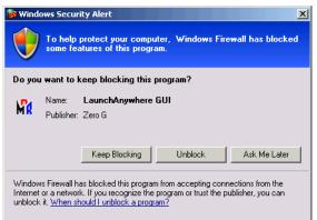
Starting NMRanalyst under Windows XP may cause the shown security alert. A similar security alert may result from starting the FindIt Database Manager of the NMRanalyst application. NMRanalyst communicates with NMRgraph and NMRplot through sockets to handle printing plots, displaying help information, and aborting adding user structures to the FindIt database. No network connection is ever attempted. Click [Keep Blocking], NMRanalyst continues to function properly and this popup won't show
