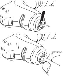
Use your fingernail or a small prying instrument to remove the lamp from the ophthalmoscope head base.
