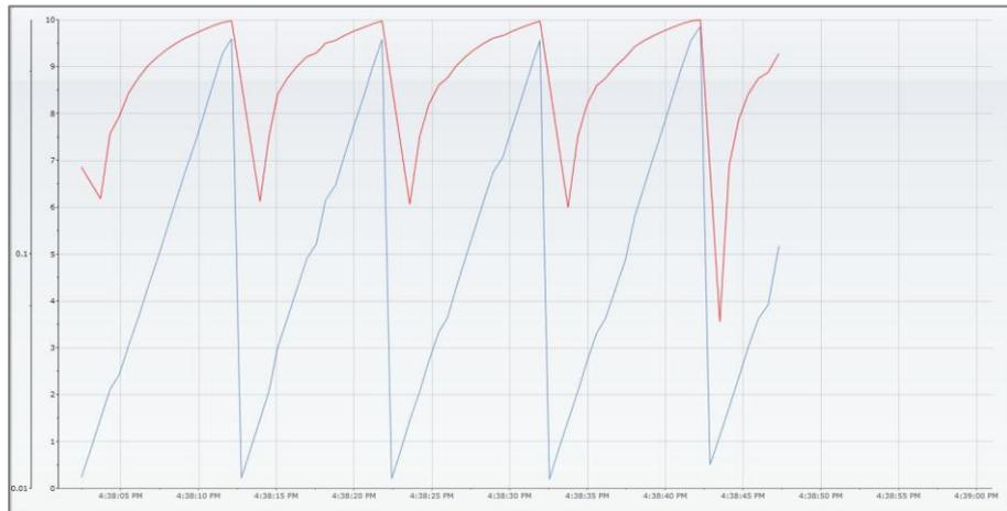
\*The same signal represented on a normal scale (blue) and on logarithmical scale (red)
