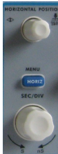
Fig. 4-13 Horizontal Control Zone
