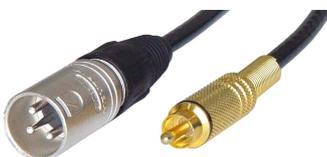
This cable is used to adapt the impedance and unbalance of digital SPDIF outputs to balanced 110  $\Omega$  AES/EBU Inputs, allowing the PAS-8 inputs to be connected to unbalanced coaxial inputs. Balancing and impedance are converted to standard AES/EBU values without any format conversion taking place. Please note that the receiving device needs to be able to process the transmitted format. The cable is usable for sample rates up to 192 kHz. Available lengths: 0.5, 1.0, 2.0 and 3.5 m.
