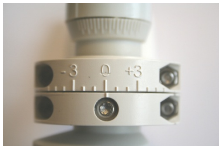
LNB in position 0
