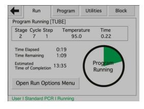
The Current Program is the one named in the status bar at the bottom of the touch screen. A program listed here is considered to be "Loaded". When "**Start Current Program**" is selected, the loaded program begins immediately, and the word "Running" appears to the right of the program name at the bottom. This run status field will also show if the program is in lid heating or holding mode.
