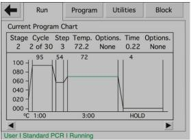
A line graph spanning the entire chart shows the Temp vs. Time at any given point. The running step will be represented by a green line segment, while the rest of the graph will be represented in black. For stages containing multiple cycles; the green line cycles through the same portion of the chart.
