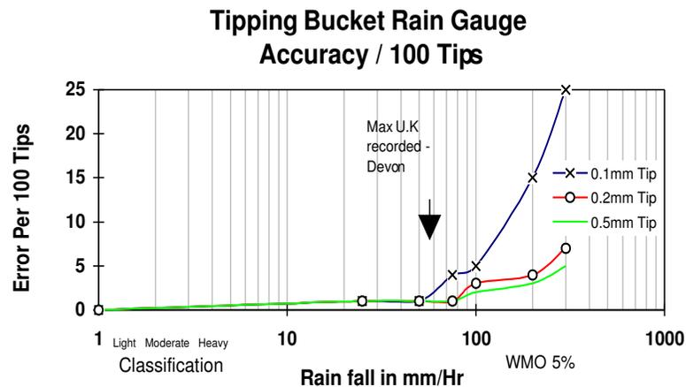
Figure 2: Accuracy of 0.1 mm, 0.2 mm and 0.5 mm tip versions
