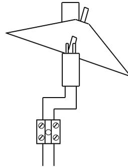
Figure 5: Connections for reed switch
