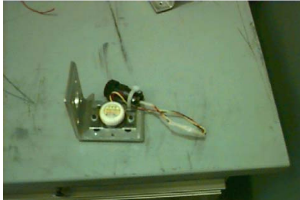
Figure 7-9. Accelerometer mounted to testing plate
