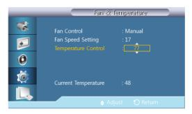
Detects the product's internal temperature and specifies the desired temperature.
