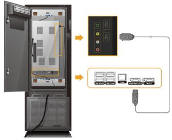
Connect the [MAGICINFO OUT] terminal of the network box and the [HDMI IN 2 (MAGICINFO)] terminal of the monitor using the **DP** to **HDMI** cable.
