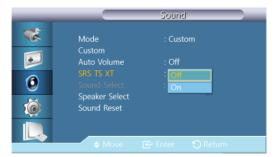
**SRS TS XT** is a patented SRS technology that solves the problem of playing 5.1 multichannel content over two speakers. TruSurround XT delivers a compelling, virtual surround sound experience through any two-speaker playback system, including internal television speakers. It is fully compatible with all multichannel formats.
