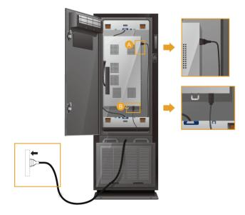
Connect the power cables inside the product to power input port  $\bigcirc$  on the product and power input port  $\bigcirc$  on the network box respectively.
