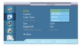
The LCD Display has four automatic picture settings ("**Dynamic**", "**Standard**", "**Movie**" and "**Custom**") that are preset at the factory.
