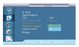
Dynamic Contrast automatically detects the distribution of the visual signal and adjusts to create an optimum contrast.
