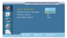
When the **Source AutoSwitch** is **On**, the display video source will automatically be searched for active video.
