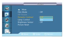
**Dynamic Contrast** automatically detects the distribution of the visual signal and adjusts to create an optimum contrast.
