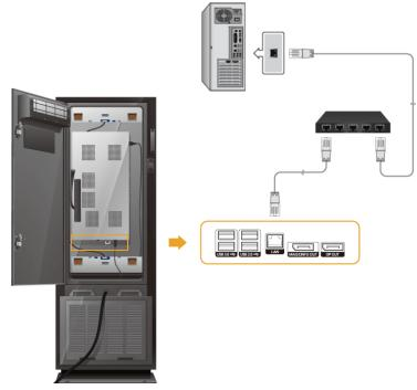
Connect the [LAN] port on the product and your network using a LAN cable.
