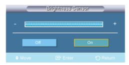
**Brightness Sensor** detects the surrounding light intensity and automatically optimizes the screen brightness accordingly.
