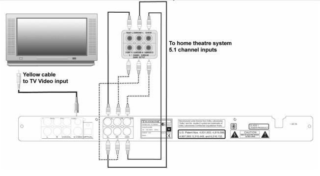
\*\* **! NOTE: 5.1 CHANNEL:** To use 5.1 Channel sound you must enter the SETUP menu and the AUDIO menu then scroll down to DOWNMIX and select 5.1 CHANNEL output.
