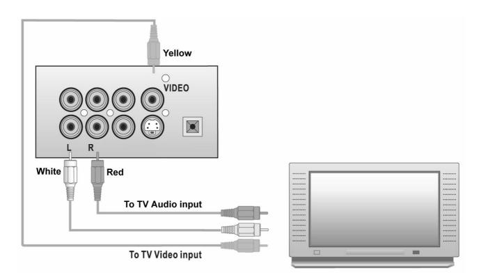
**DVD Connections:** Connect the Yellow plug to the Yellow Video output jack Connect the Red plug to the Red R (Audio Right) output jack Connect the White plug to the White L (Audio Left) output jack
