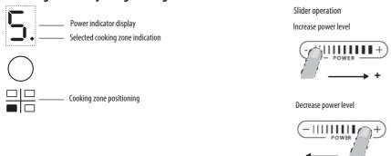
After switching the hob on, activate the required cooking zone by pressing the corresponding circular button and place the pot on the zone. With the Slider control it is possible to select the required power level, from min. 0 to max. 9, or booster "P" if available.
