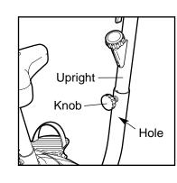
ment holes in the upright with the indicated hole in the frame. Insert the knob into the frame and the upright, and turn the knob clockwise until it is tight. Make sure that the knob is inserted through one of the adjustment holes in the upright.
