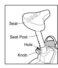
slide the seat post up or down and align one of the adjustment holes in the seat post with the indicated hole in the Frame. Insert the knob into the frame and the seat post, and turn the knob clockwise until it is tight. Make sure that the knob is inserted through one of the adjustment holes in the seat post.
