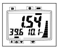
will then show only the elapsed time, and the lower left section of the display will show only the number of calories you have burned. Press the Mode button again. The upper section of the display will then show only the distance pedaled, and the lower left section of the display will show only the number of fat calories you have burned. To select the scan mode again, press the Mode button repeatedly until a mode bar appears below the scan symbol.
