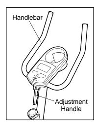
wise, push it toward the handlebar, and then turn it counterclockwise. Repeat this procedure until the handlebar is loose.) Rotate the handlebar up or down to the desired position, and then turn the handle clockwise until it is tight.
