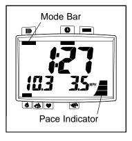
the distance that you have pedaled; the lower left section of the display will alternately show the number of calories you have burned and the number of fat calories you have burned; and the lower right section will show your pedaling speed.
