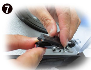
3 Separate the cartridge from the socket lightly.
