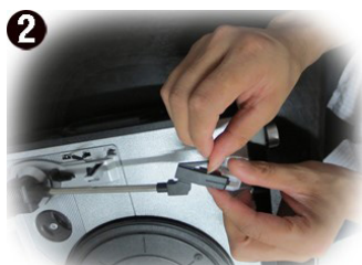
2 Remove the plastic cap to access the stylus.
