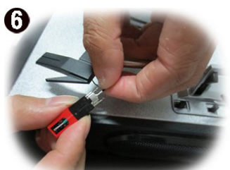
2 Remove the plastic cap to access the stylus.
