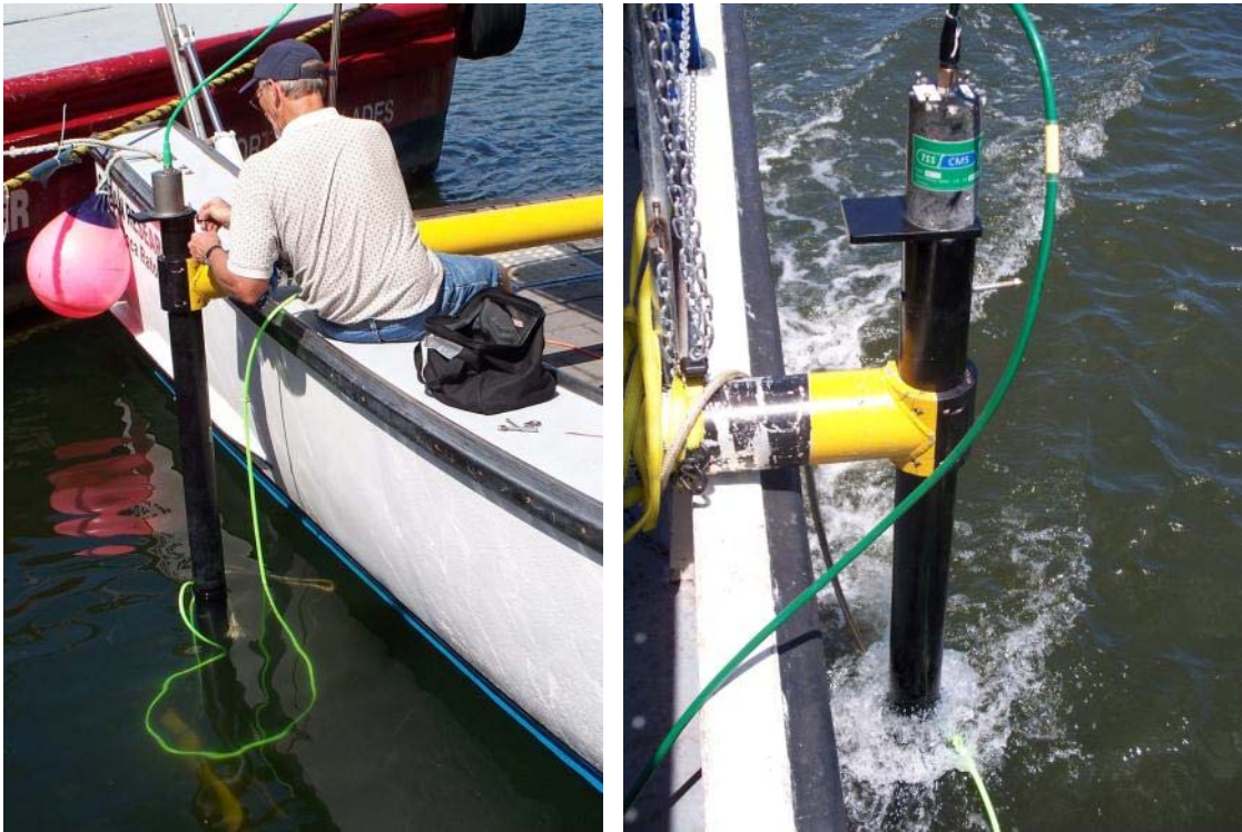
Figure 10: 4600 Deployment, Option 2: Over-the-Side
