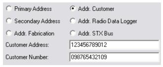
The customer addressing mode uses a 12 digit customer address and a 12 digit customer number to address the device. Very few devices are supporting this addressing mode.
