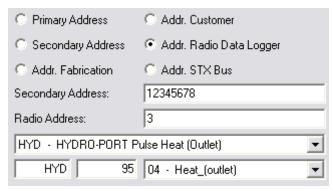
The radio data logger addressing mode is used if there are radio data logger with M-Bus connections installed. The radio data logger have got an internal primary address in the range of 0 to 250 which must be entered at the appropriate field. The other parameters are the same as for standard secondary addressing.
