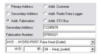
The secondary addressing mode with the 8 digit fabrication number is similar to the standard secondary addressing, except that the fabrication number is also used. Very few devices are supporting this addressing mode.
