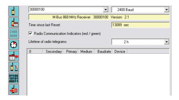
Apart from the serial number and the baudrate, the firmware version and the time in seconds from the last restart of the M-Bus radio receiver are shown. The radio communication indicators (green and red LED, blinking for a successfully or an erroneously received radio telegram) may be switched on or off.
