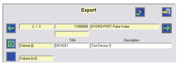
6. You may now select the meter values to export by checking or un-checking the blue buttons on the left hand side of the meter value descriptions. Additionally, you have to enter a unique TAG ID and
