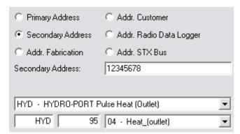
The standard mode is Secondary Address where the 8 digit serial number of the device and its device type parameters (manufacturer code, generation code, medium code) are used to address it. Fill in the serial number as secondary address and select a device type from the list of known devices.
