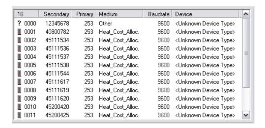
The leftmost column contains the number of the radio device, the other columns containing the secondary address, the primary address (always 253 since it is only virtual), the measured medium, the baudrate and the device type.
