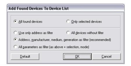
First of all you may add all found devices or only the devices selected to the main device list. After that you may also opt for comparing the found devices and the devices already in the main list. Depending on the filter option, all devices, only devices with different serial number (address), only devices with different serial number (address) and different device type (manufacturer, medium, generation), or only devices which are completely different are added to the main device list.
