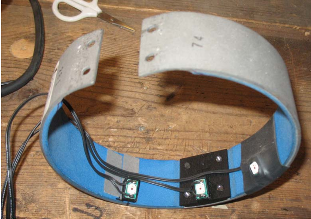
Figure 13. Cable routing for rearward and center LEDs
