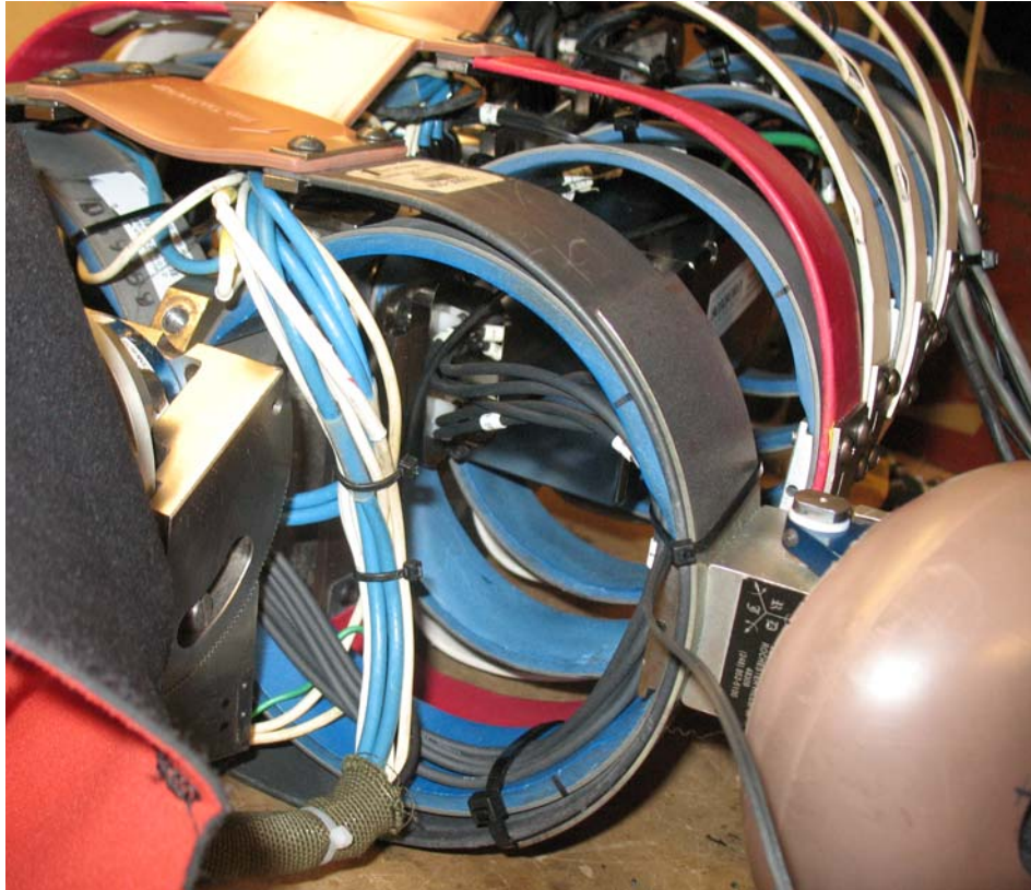
Figure 27. Sensor cables tied to controller
