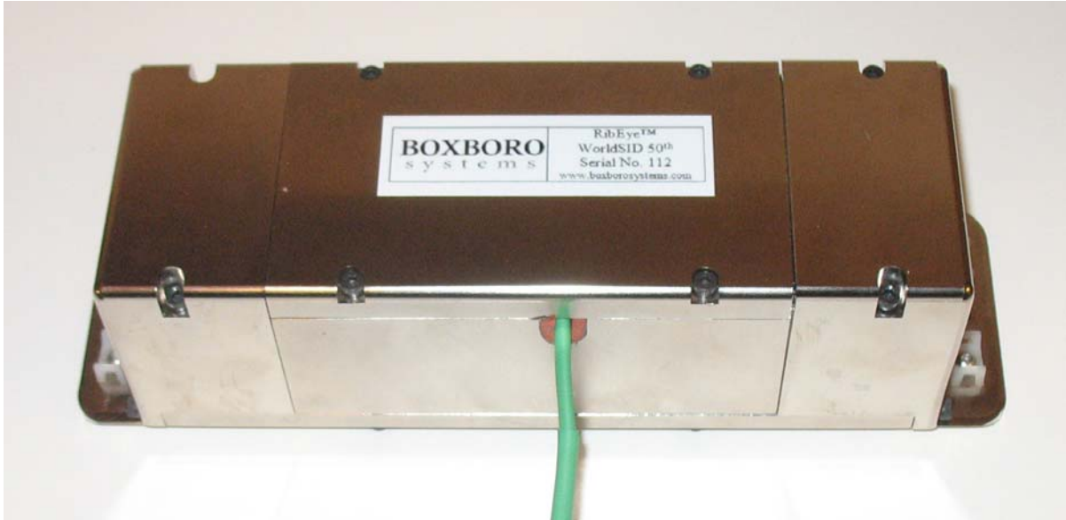
Figure 3. RibEye controller with connector covers in place (green cable exiting from DAS battery pack)
