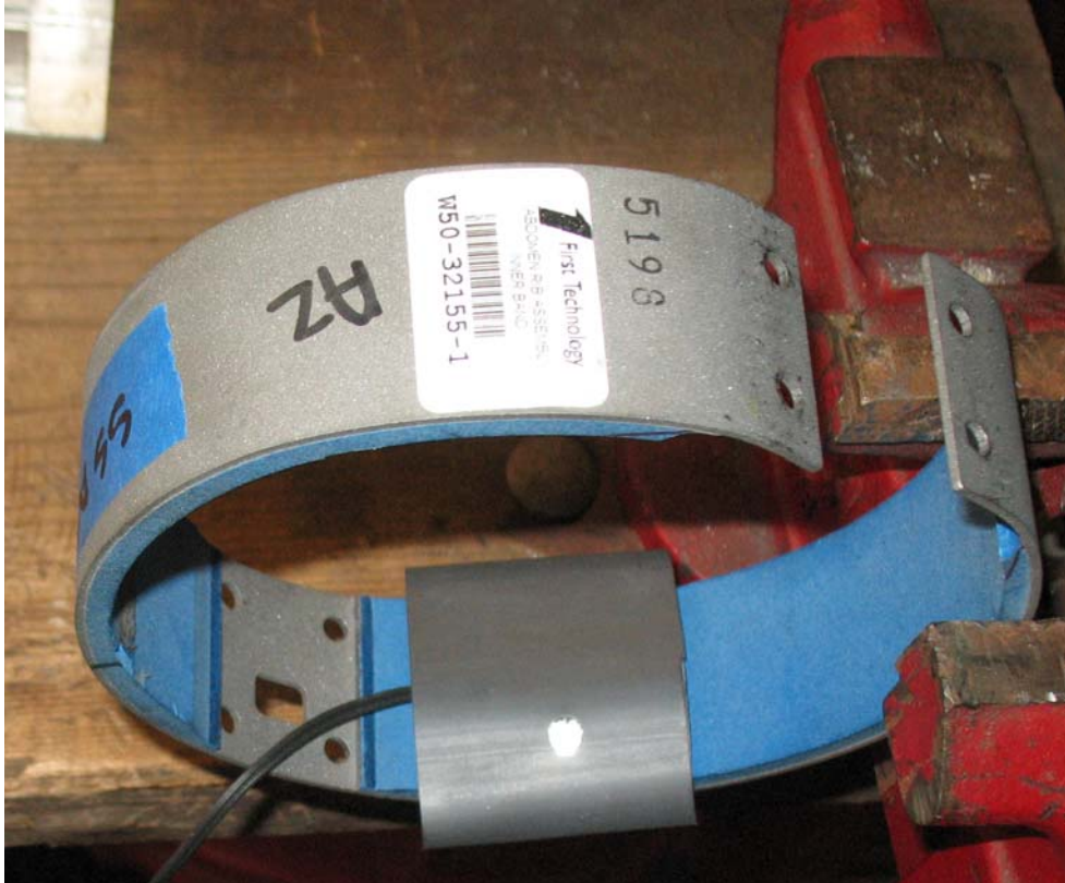
Figure 12. Heat-shrink tubing placed over rearward LED
