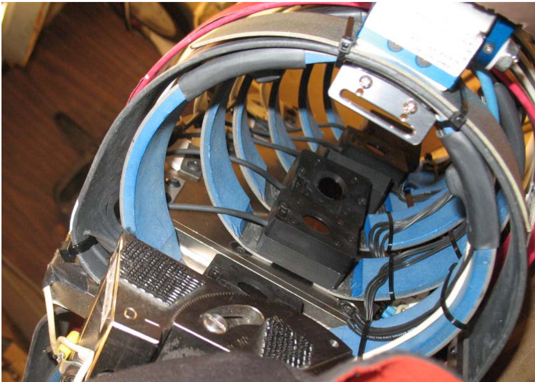
Figure 24. Sensor cables routed to back of dummy
