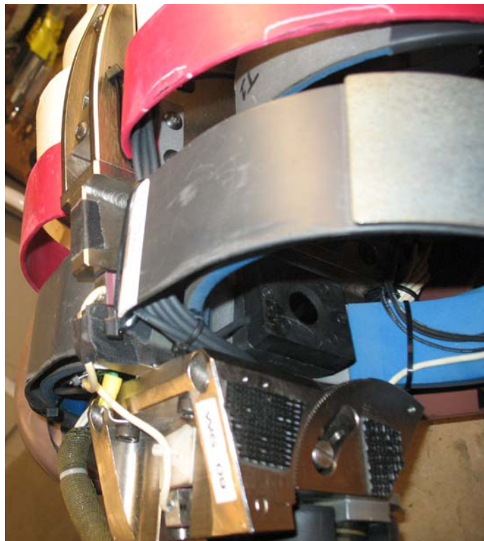
Figure 26. Sensor cables routed over the top sensor and below the neck assembly
