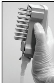
17. Whilst the tool is held over the PyroMark Q24 Plate, close the vacuum switch on the tool (Off).
