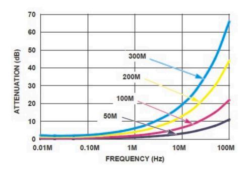
In order to transmit the VGA over CAT-5, differential signal transmission is considered for almost all of VGA over CAT-5 extenders. Because of the low bandwidth of the cables, on the receiver is inevitable. Appropriate compensations such as equalization and gain control, and even delay adjustment among component colors are a necessary means in order to get at least acceptable quality of video and audio.
