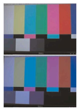
Color mismatch is the effect of a difference in gain or offset of the color channels. Example shows the screen on the bottom has excess blue.
