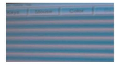
Power supply noise appears as a repetitious disturbance in the video picture. Use a higher quality voltage regulator to power the amplifiers and bypass all chipsets as close to the power pins as possible.
