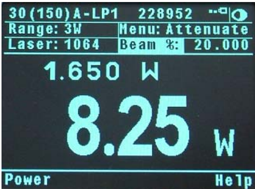
Figure 4.8 Attenuation Screen with Beam % set to 20%
