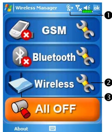
❶ This icon will show up on your screen whenever your Pocket PC has detected a usable wireless network and has connected to that network, indicating that your Pocket PC has successfully connected to the network hotspot (Access Point). At this point, the indicator on the upper left of your Pocket PC will flash orange.
