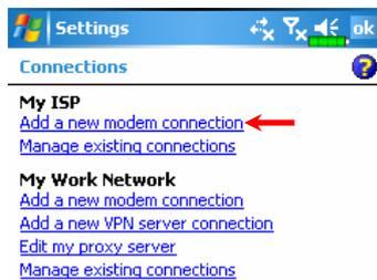
1. As shown in the screen on the left tap “Add a new modem connection.”
