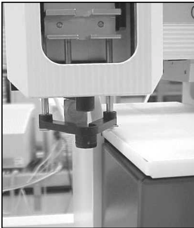
Figure 3. Injection unit in the “FiberExp” position with the right edge just touching the left rear edge of the agitator.
