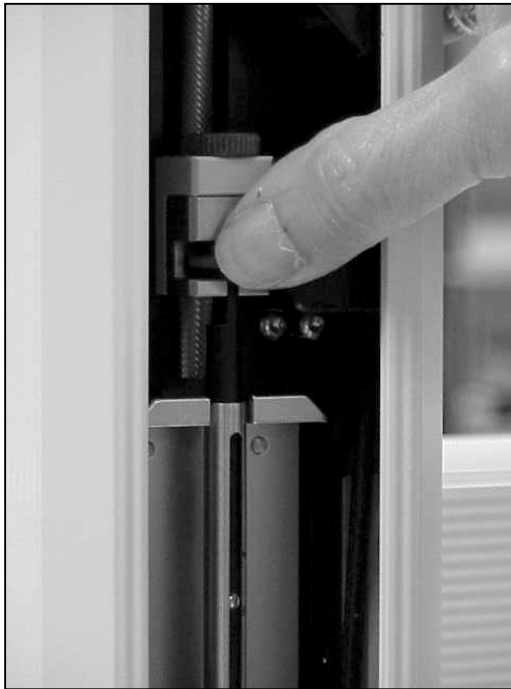
Figures 5A and 5B. Installation of the fiber adapter in the Combi PAL injection unit
