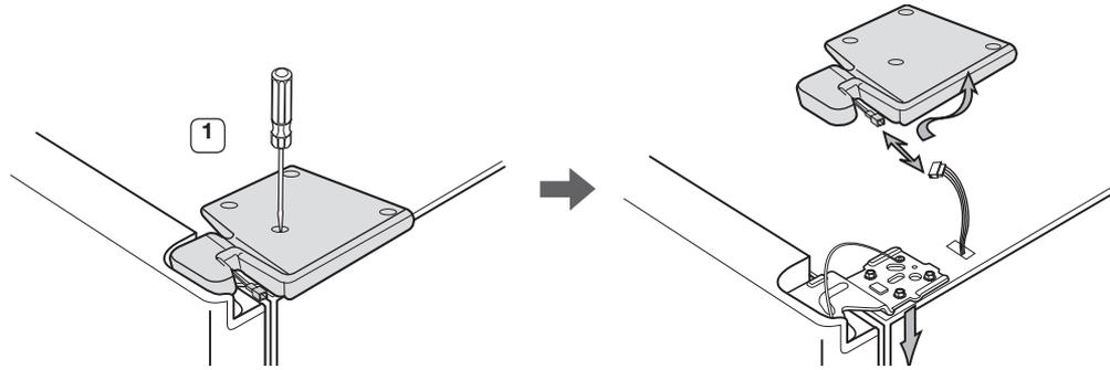
2. Remove hinge screws **2** and the ground screw **3** by turning counter-clockwise, and take off the upper hinge **4**. Be careful that the door does not fall on you as you are removing it.
