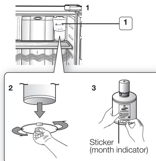
4. Remove the filter cap and insert the filter into the filter housing.
