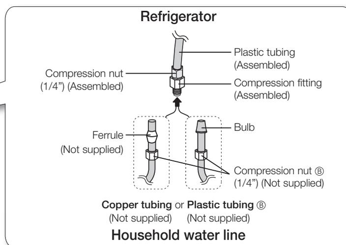
1. Connect the household water line to the assembled compression fitting.
