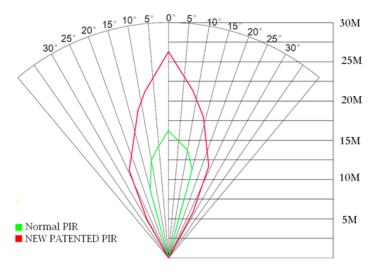
The PIR detection angle ( $\alpha$ ) is just smaller than the field of view (FOV) angle ( $\beta$ ). The advantage of this design is to reduce empty picture rate and capture most, if not all, motions.
