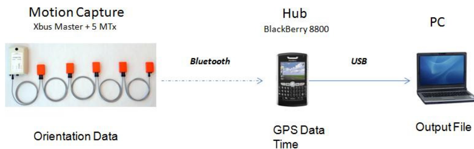
Figure 5.1: System architecture for the preliminary testing.
