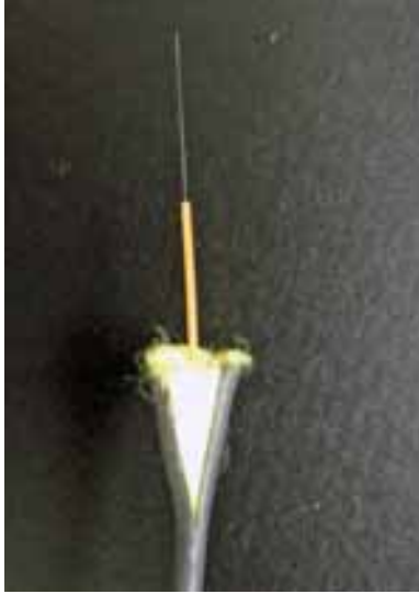
Figure 2: Slit Cable with Stripped Fiber
