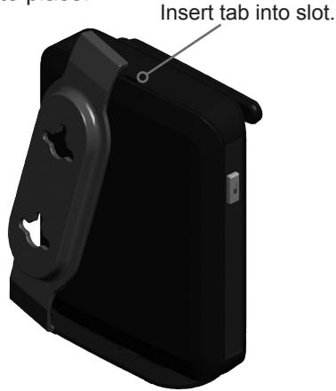
4. Check to make sure the plate is secure at top and bottom. It should be flush with the base station body.
