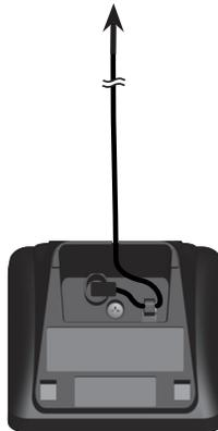
Plug the power adapter into an electrical outlet not controlled by a wall switch.
