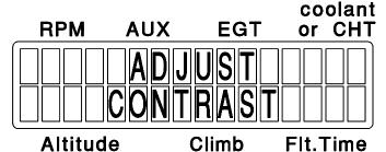
shut the instrument off then turn it on again. The newly stored contrast setting will remain in effect and you can then press the Lmts button while the introduction is rolling in. A taller or shorter pilot may have to readjust the contrast as a result of the different viewing angle. Also, temperature affects the contrast somewhat and it may require adjustment if subjected to a significant temperature change.
