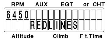
The RPM redline value is displayed and can be changed with the up/dn switch. Pressing the Lmts pushbutton then advances to the next redline item. Note that once you press the Lmts switch to move forward, you can't go backwards. If you skip by a desired redline item, you will have to turn the instrument off and on again and start all over.
