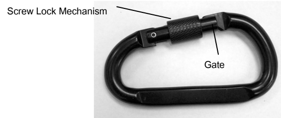
1. Carabineer with Gate closed but Screw Lock Mechanism Open
