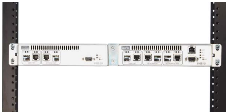
Figure 3-7 Two 9145Es Mounted on Rack
