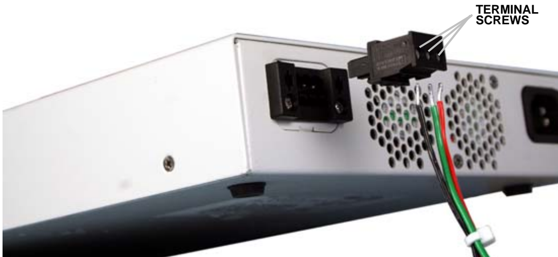
Figure 3-11 Connect D.C. Power
