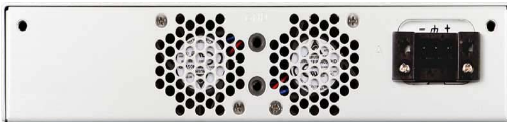
Figure 2-6 Single DC Power
