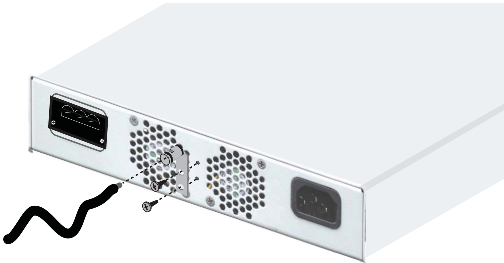
Figure 3-12 Install Grounding Lug
