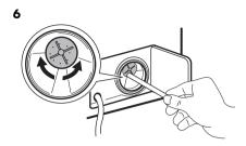
Use a pencil to check whether the pump wheel right at the back of the pump housing can turn. (It is normal for the pumping wheel to turn jerkily.) If the pumping wheel cannot be turned, please contact the After Sales Service.
