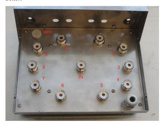
On the bottom side the antenna connectors are located according to the pictures above. The antenna switch is normally delivered with SO-239 jack but can also be ordered with N connectors. The ventilator will prevent moisture to build up in the housing.
