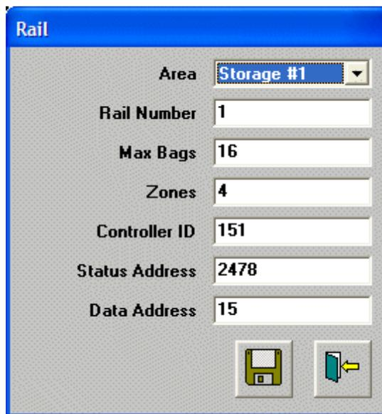
Each rail needs to have an area assigned. See the diagram on page 6 for reference when assigning these areas. A rail number is also needed, as well as the maximum number of bags the rail can hold. **Note that rails always begin at number one.** Although the user sees Storage Area rails starting at 101, they start at 1 internal to the program and controllers.
