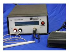
5. Attach the Electrode tip to the Electrode Cable, gently slide the electrode tip onto two pronged end of the electrode cable and secure gently.
