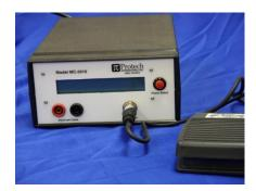
4. Plug the Electrode cable into the front of the box where indicated.
