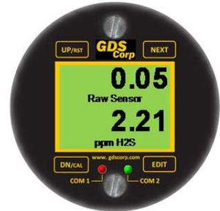
Below the LCD display, two LEDs monitor the MODBUS RS-485 or Ethernet network interface. Flashing indicates sent or received data.
