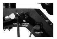
Connect camera power and video cables to the camera.
