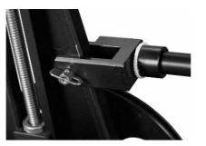
Start with the base rod at the crane pivot. Make sure the rod end is mounted as shown.
