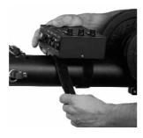
Mount the control box close to the end of the counterweight rod on to the crane tube with the Velcro straps and the connectors facing the top of the crane.
