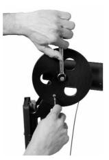
To remove the disc, loosen and remove the hexagon socket screw using the 4 mm Allen wrench.
