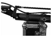
Use an apple box or a shipping case to keep the crane and head off the ground.
