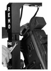
Depending on the camera size (length) the height of the remo one head can be adjusted.
