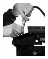
Connect the slave cable to the main cable and slide it through the center hole in the head.
