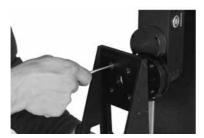
Attach the Remo head adapter to the top of the head with 6 screws.
