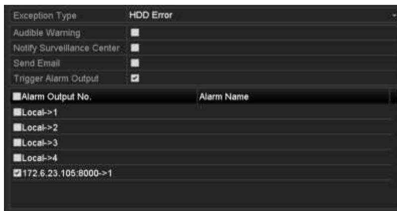
Figure 10. 23 Configure HDD Error Alarm
