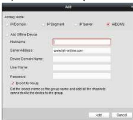
Figure 9.13 Access Device via iVMS-4200
