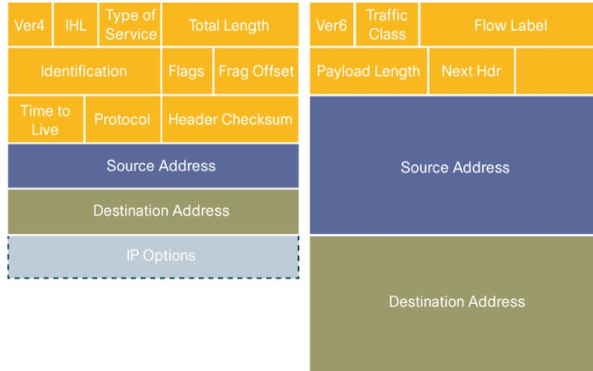
Figure 3.1. IPv4 and IPv6 headers [5]
