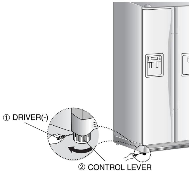
Case 2) Freezer door is higher than that of the refrigerator
