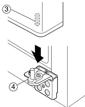
3) Insert the upper hinge shaft (⑤) into the hole (⑥). After levelling between the upper hinge hole (⑦) and the hole of the cabinet (⑧). Reattach hinge screws (⑨) and ground screw (⑩) in the clockwise direction.
