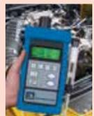
**Kane Five (5) Gas Analyzer is a Hand Held Portable Tester Powered by 110V or Internal Rechargeable Battery Pack**
